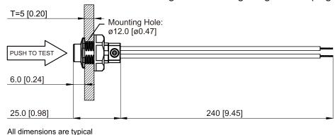
Dimension unit: mm [inch] Tolerance: ±1 [0.04]
